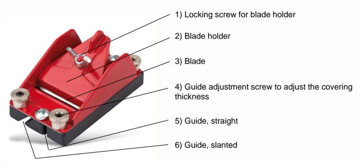
To-and-fro movements of the loose blade holder (2) adjust the blade (3) to the required cutting depth.
